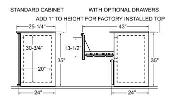
Note: Available with compressor left or right. Compressor left model shown.
